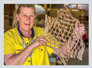
Waste cardboard is now perforated and used as a substitute for plastic bubble wrap, effectively eliminating two problem wastes.
