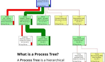
A **Process Tree** is a hierarchical representation of the processes in the life cycle of a product, the thickness or colour of the flow lines are used to depict the amount of impact.
